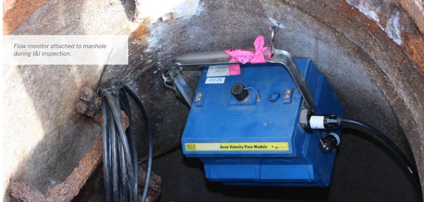
Flow monitor attached to manhole during I&I inspection.
