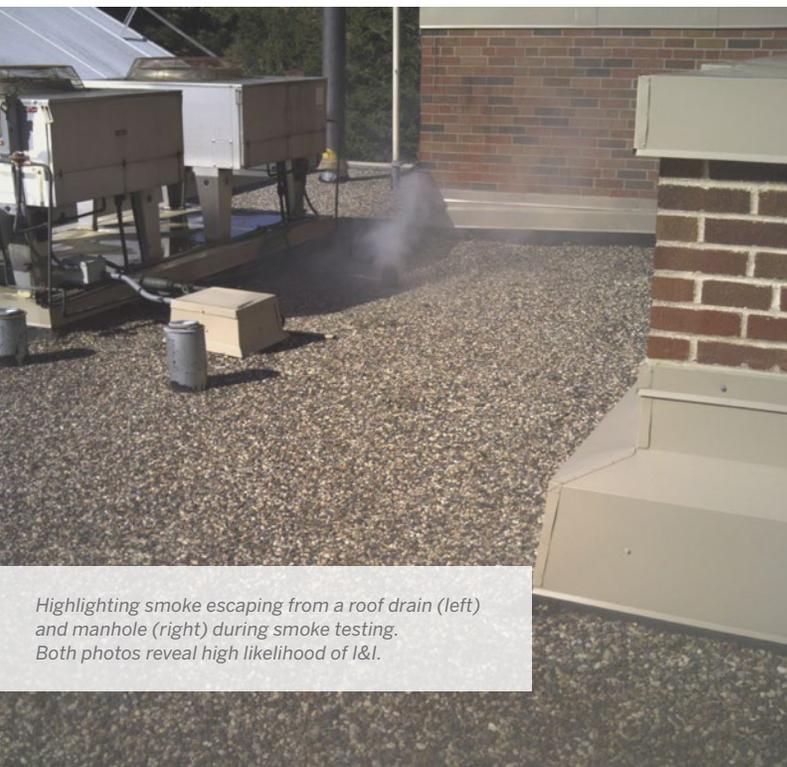
Highlighting smoke escaping from a roof drain (left) and manhole (right) during smoke testing. Both photos reveal high likelihood of I&I.
